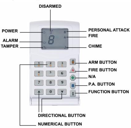
Whilst the keys and displays for both keypads differ, their functionality is very similar. Where functionality differs, methods for both keypads will be described. Where functionality for both keypads is the same, only one set of instructions for both are described.
