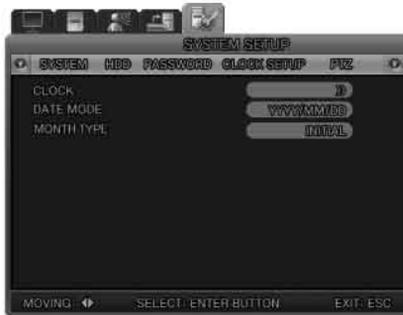
· CLOCK : Set the system time. The unit will automatically reboot for system stabilization.
