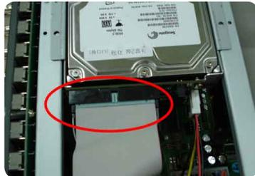
Connect to the E-IDE HDD cable
