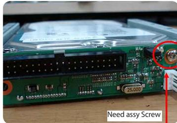
3. Select "Master" or "Slave" using the Jumper switch on SATA converter board.
