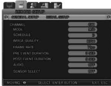
· CHANNEL : Select the channel for which to set DETAILED SETUP.
